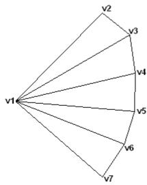
The system uses vertices v2, v3, and v1 to draw the first triangle, v3, v4, and v1 to draw the second triangle, v4, v5, and v1 to draw the third triangle, and so on. When flat shading is enabled, the system shades the triangle with the color from its first vertex.
