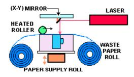
Sheets of paper or plastic film are attached to previous layers by either sprayed glue, heating, or embedded adhesive, and then the desired outline of the layer is cut by laser or knife. Finished product typically looks and acts like wood.
