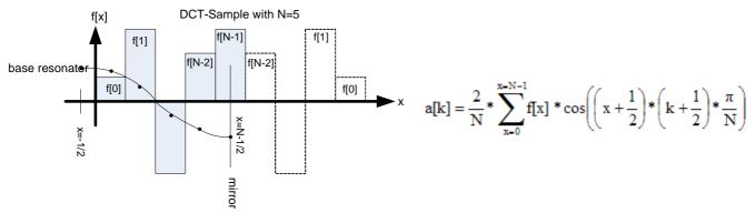
The code lenght of the DCT algorithm is much shorter than the correponding DFT code (but execution time remains identical):
