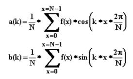
Since we need  $\mathbb{N}$  cosine- and  $\mathbb{N}$  sine-resonators, we prepare the resonators in a suitable way in form of a quadratic  $\mathbb{N}*\mathbb{N}$ -cosine-matrix and a sine-matrix of the same size.
